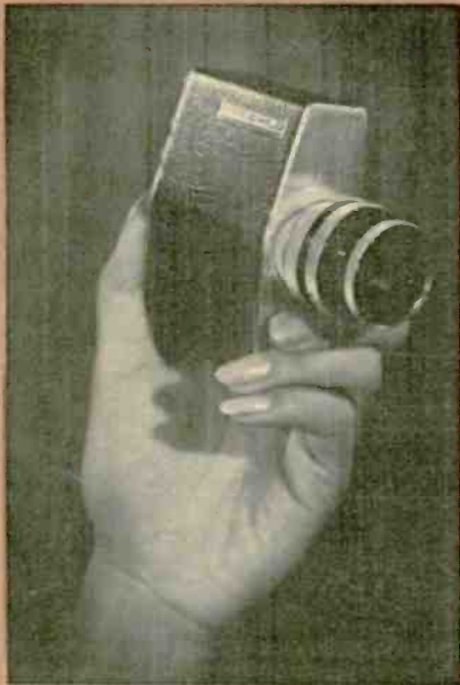
FAIRCHILD MV-100 TV CAMERA measures 3\frac{1}{2} x 1\frac{1}{2} x 2\frac{1}{4} inches (without lens) and weighs 6 ounces. It operates over a wide range of light levels and its power consumption is low.
